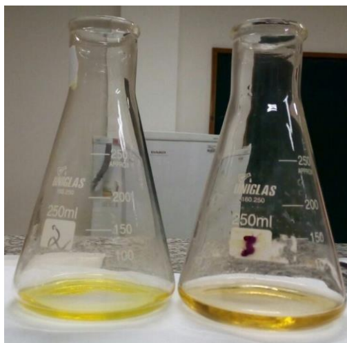
Figure 4- HCl solution titrated with [\text{NaOH}] = 0,09724 \text{ mol L}^{-1} employing CUR as an indicator before (left) and after (right) the titration end point.
