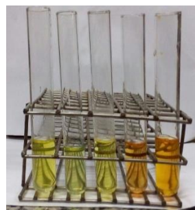
Figure 3- Color variation of CUR as a function of pH. Observations from left to right pH=1; 2; 6; 10 and 14.
